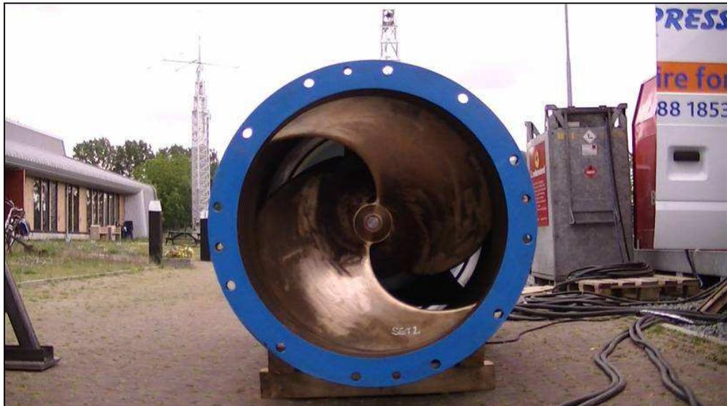
figure 1.1 *Impeller of Bedford pumps SAF.90.05.12.*
